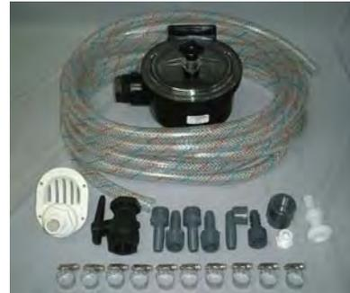
Included in the kit is a seawater inlet thru hull with a speed scoop, ball valve, seawater strainer, overboard thru-hull, 25' of hose, hose clamps and necessary PVC fittings to complete the average installation. See Aqua-Air<sup>®</sup> brochure "Seawater Kits / SWK Series" #80625 for a complete description of all of the components included in these kits.
