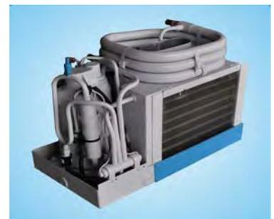
The **mini-kool** unit is commonly used in new installations however it is very well suited to the replacement or retrofitting of an older, less efficient or obsolete unit, or as an upgrade. This self contained unit is a refrigerant to air heat exchanger that has all the major components mounted on one chassis. It is installed in the area of the boat that is to be heated or cooled.
