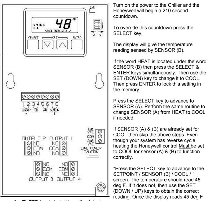
press the ENTER key to lock this setting into the memory.
