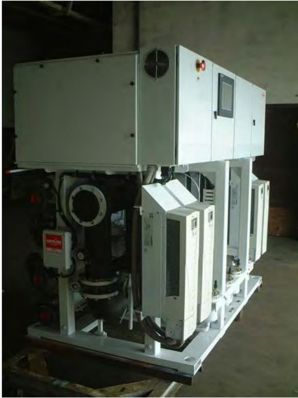
The unit is also equipped with a highly innovative Manual Bypass System for the PLC which allows the crew to still control the chiller in the unlikely event that there is a catastrophic failure of the touchscreen or PLC. You can see more pictures and read a complete specification on our website
