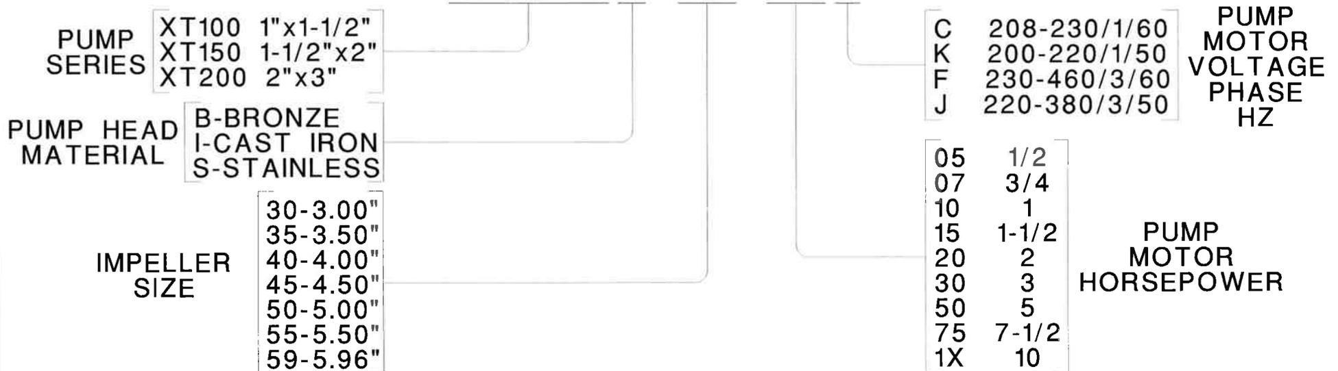
THE EXAMPLE ABOVE IS A XT150 SERIES PUMP HEAD, BRONZE CONSTRUCTION, 4.50" IMPELLER 7-1/2 HP MOTOR CAPABLE OF RUNNING ON EITHER 230 or 460 VOLT 3 PHASE, 60 HZ.
