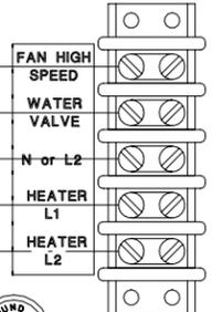
TERMINAL STRIP FOR ALL AQH, AQP & AQV FAN COILS WILL BE LOCATED ON THE BLOWER MOTOR TRAY.
