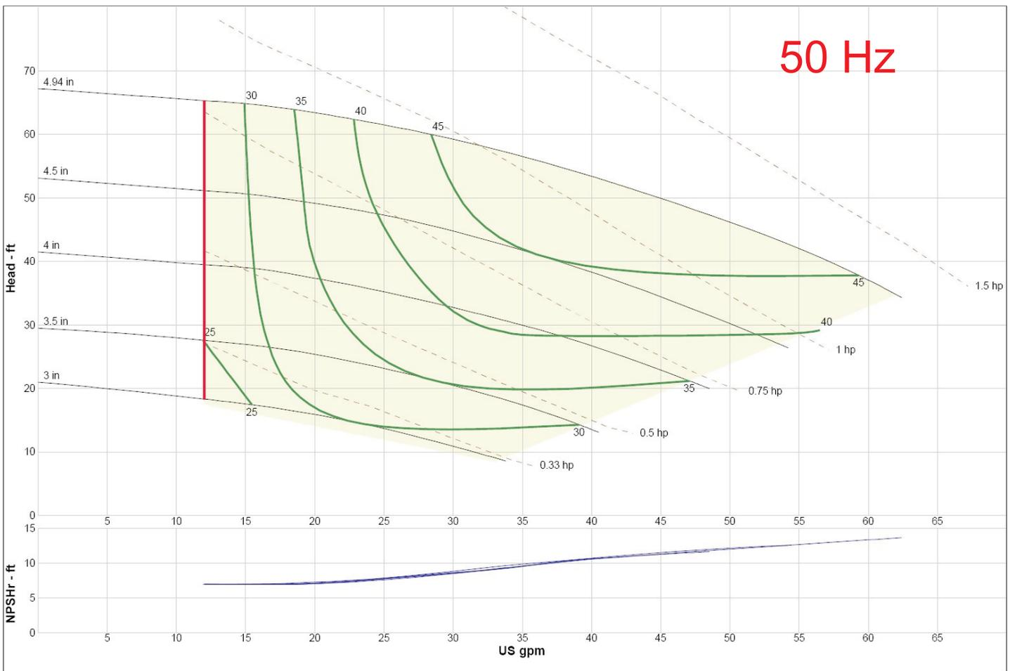
The XT Series Centrifugal Pump is available in bronze for seawater use, cast iron for chillwater use or stainless steel for special applications. Motors are available for all voltages, 50 and/or 60 Hertz, single or three phase. The standard motor style is TEFC (Totally Enclosed Fan Cooled). The ODP (Open Drip-Proof) style motor is available on special order. Flow rates up to 400 GPM and 160 feet of head are possible with this series of pumps.
