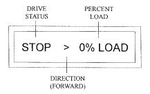
Pressing the ENTER key again will change the display from the % LOAD indication to the VAC (motor voltage) indication:
