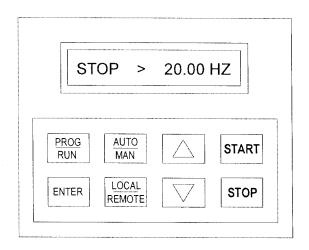
To program the drive, the PROGRAM mode must be entered by pressing the PROG/RUN button. If the password protection is disabled, pressing the PROG/RUN button will result in direct entry into the PROGRAM mode. If the password protection is enabled, the PASSWORD prompt will appear when an attempt is made to enter the PROGRAM mode. The PASSWORD prompt appears as follows:
