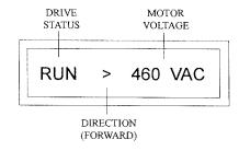
**NOTE:** During acceleration and deceleration to the SPEED SETPOINT, the DRIVE STATUS will show the actual drive speed. When the SPEED SETPOINT is reached, the DRIVE STATUS will change to RUN (or STOP if the drive is decelerating to a STOP).
