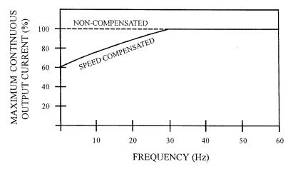
The "speed-compensated" thermal overload circuit offers additional protection from high load conditions at low speeds, where motor cooling is often less effective (e.g., motors with shaft-mounted fans). As seen on the diagram below, the drive reduces the allowable continuous output current when operating at frequencies less than 30 Hz.
