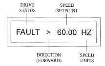
**NOTE:** To clear a FAULT, press the STOP key, issue a remote STOP command at TB-1, or use TB-13D (refer to Parameter 50 - TB13D).
