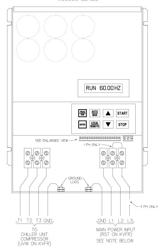
NOTE: FOR SINGLE PHASE INPUT CONNECT POWER TO L1 AND L2. ENSURE THAT A JUMPER IS INSTALLED BETWEEN L2 AND L3.
