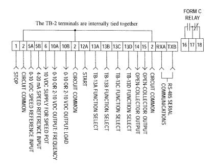
**NOTE:** The function of terminals TB-10A, TB-10B, TB-13A, TB-13B, TB-13C, TB-13D, TB-14, TB-15, TB-16, and TB-18 are dependent on the programming of certain parameters. In most cases, the name of the parameter matches the number of the terminal, allowing quick and easy programming of the terminals to suit the application. The exception is TB-16 and TB-18, which are governed by Parameter 54 - RELAY.
