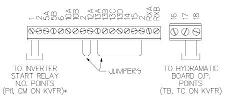
\* THESE TWO WIRES MUST BE CONNECTED TO THE COMMON AND NORMALLY OPEN POINTS AT THE RELAY.
