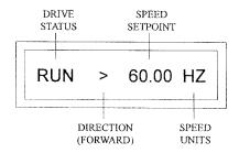
As in the STOP mode, the ENTER key can be used to toggle the display from SPEED to % LOAD to VAC (motor voltage):
