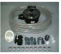
Included in the kit is a seawater inlet thru hull with a speed scoop, ball valve, seawater strainer, overboard thru-hull, 25' of hose, hose clamps and necessary PVC fittings to complete the average installation. See Aqua-Air<sup>®</sup> brochure "Seawater Kits / SWK Series" #80625 for a complete description of all of the components included in these kits.
