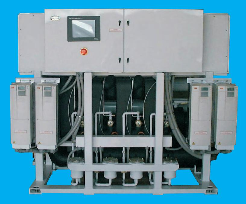
A60P4-VIHD 60 Ton (720,000 BTU/H) 4 Stage, Semi-hermetic Compressors PLC / Touchscreen Control Variable Frequency Drives Integral Immersion Heater
