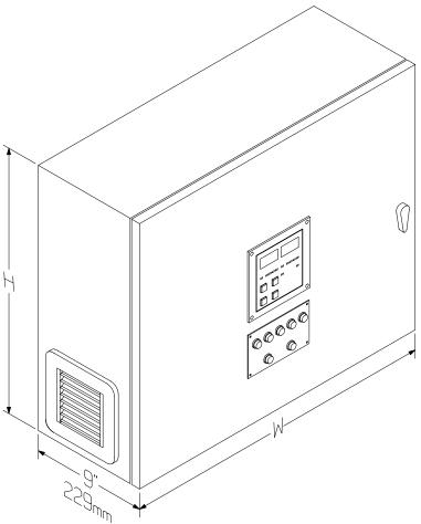
ALLOW 6" (150mm) ON THE LEFT. RIGHT & BOTTOM OF THE ELECTRICAL BOX FOR VENTILATION AND ACCESS TO THE ELECTRICAL CONNECTIONS AND GLAND PLATE
