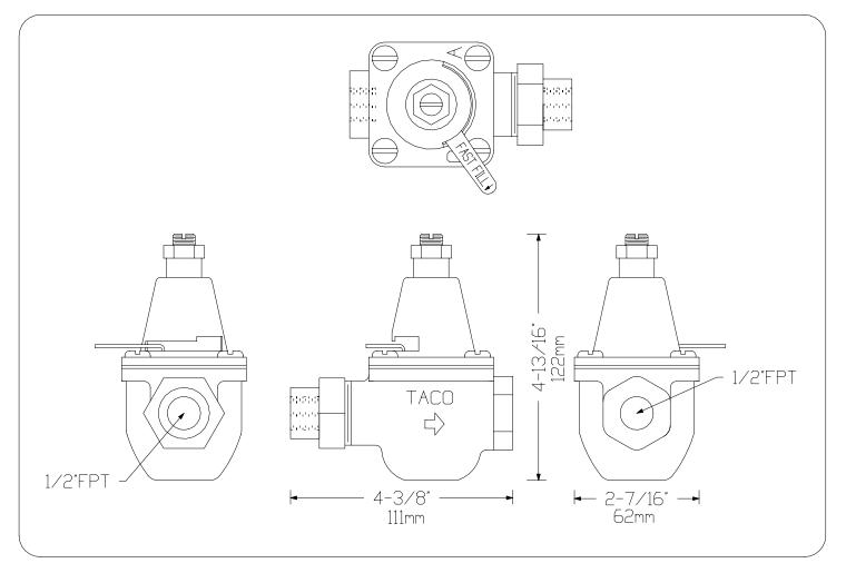
MAXIMUM WORKING PRESSURE: 100 PSIG FACTORY OUTLET PRESSURE SETTING: 12 PSIG OUTLET PRESSURE SETTING RANGE: 5-25 PSIG MAXIMUM WORKING TEMPERATURE: 212°F / 100°C WEIGHT: 2.2 LBS / 1.0 KG
