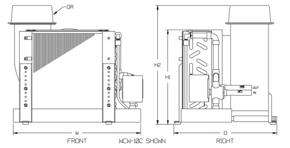
Model Number Examples Unit without Internal Element Heater WCW-16C 16 = 16,000 BTU/HR C = 230-1-50/60
