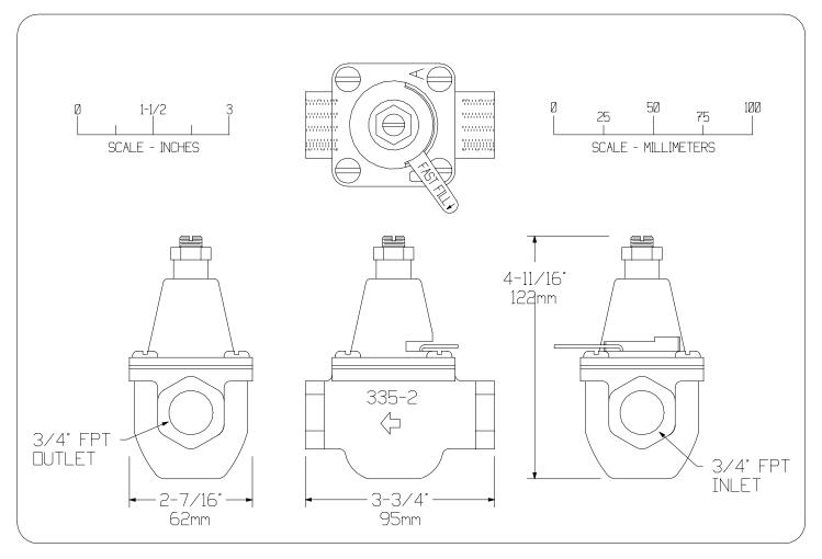
MAXIMUM WORKING PRESSURE: 100 PSIG FACTORY OUTLET PRESSURE SETTING: 12 PSIG OUTLET PRESSURE SETTING RANGE: 5-25 PSIG MAXIMUM WORKING TEMPERATURE: 212°F / 100°C WEIGHT: 3.5 LBS / 1.6 KG
