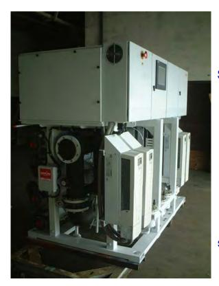
The unit is also equipped with a highly innovative **Manual Bypass** System for the PLC which allows the crew to still control the chiller in the unlikely event that there is a catastrophic failure of the touchscreen or PLC. You can see more pictures and read a complete specification on our website www.aquaair.com
