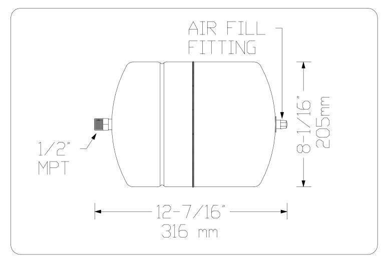
MAXIMUM WORKING PRESSURE: 100 PSIG FACTORY PRE-CHARGE PRESSURE SETTING: 12 PSIG MAXIMUM WORKING TEMPERATURE: 212°F / 100°C WEIGHT: 5.0 LBS / 2.3 KG
