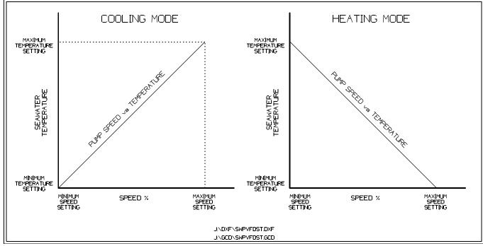
Operation of Seawater Pump VFD in Cooling and Heating (Reverse Cycle) Mode
