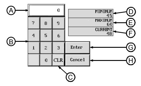
On the right side of the screen the **MINIMUM** setting (D), **MAXIMUM** setting (E) and **CURRENT** setting (F) appear.
