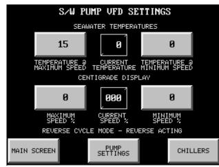
11. Seawater Pump VFD Control
