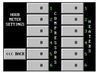
18. Compressor & Heater Hour Meter Adjustments
