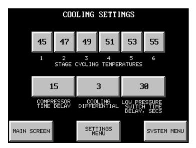
TEMPERATURES button. A numeric keypad will appear. Enter the stage temperature desired within the allowable range (see Programmable Parameters sheet) and press ENTER.
