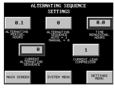
HOURS display. When the sequence changes it always moves ahead by one position. An example of this is a four compressor unit:
