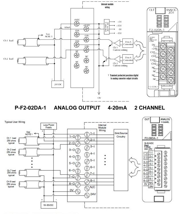
NOTE 1: Shields should be connected to the 0V terminal of the module.
